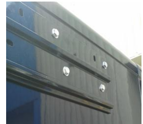
Compact Cassette securely fitted to body
