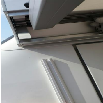
Fig 4 Caravan Rail for side sheet
