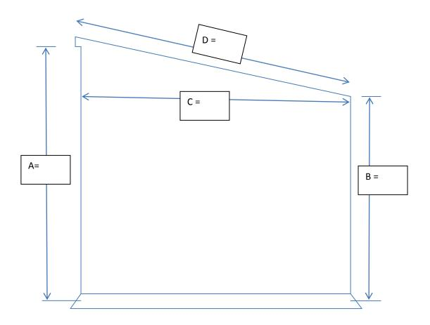
A = the ground to the underneath side of the awning cassette
